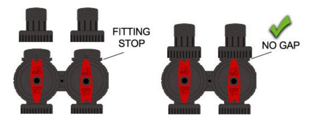
If there is a gap between the connector collar and the fitting stop, it is not threaded on far enough. Excessive force is not required to obtain a good seal. Do not over-tighten.
