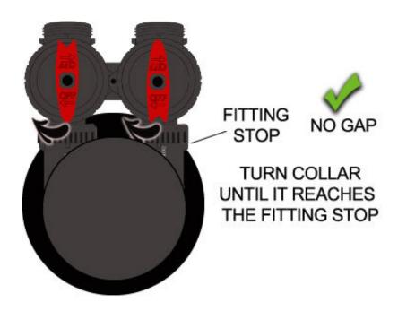
Step 6. - Connect 1" NPT Connectors to the Bypass Assembly
